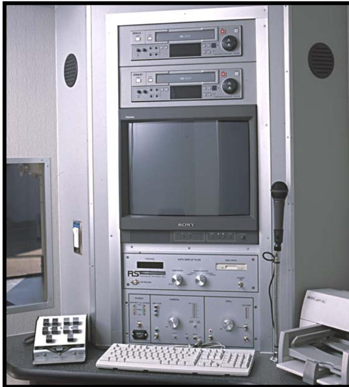
The Model 20-2000 Controller Power Supply is a component of a vehicle mounted or transportable video inspection system. The components of a vehicle system are mounted in a 19-inch standard relay rack, which is part of the operator's control console. The components of a transportable video inspection system are mounted in a 19-inch standard relay rack, which is mounted inside a 1/8" aluminum container. This container provides protection while being transported.
