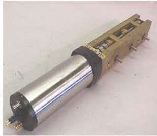
Inspect bridle, bulkhead, and camera power cable, upper skid rails and screws.
