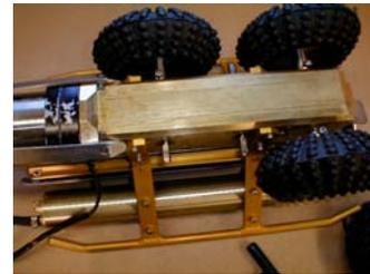
5. Install tires. Turn completed assembly upside down. Rotate all axles until the flats are pointed upward. Slide the tire assembly on the axles and tighten with an Allen wrench.
