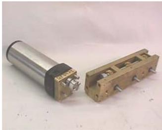
Move axles in all direction to check for excessive wear in the bushing.
