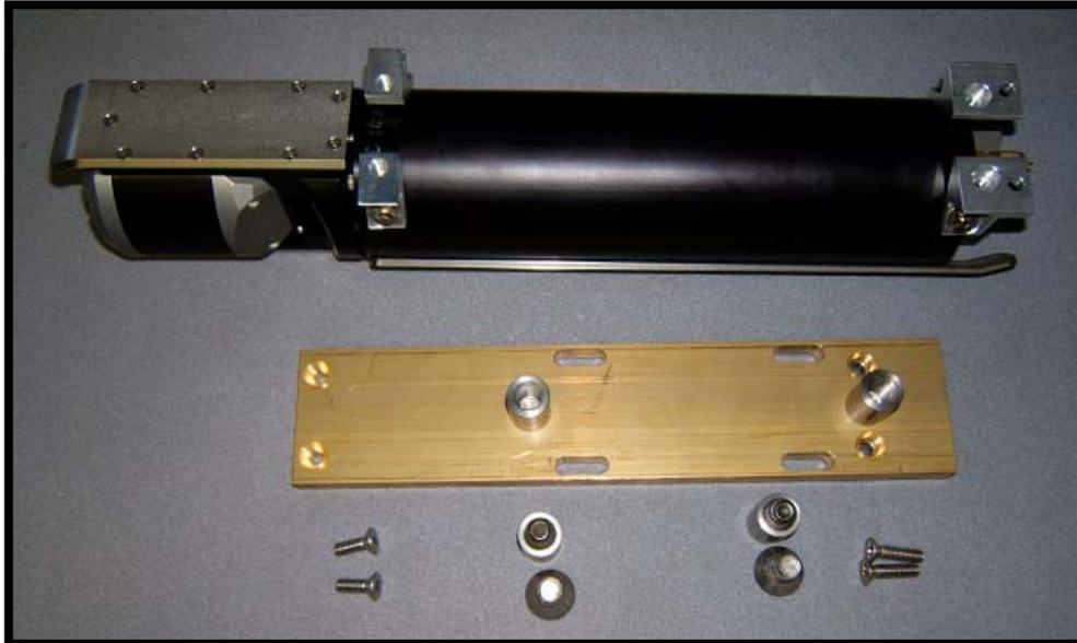
Place the camera on its back. Place the riser plate onto the camera. Use two 1/4-20 x 1" flat head screws to fasten the rear brackets to the base plate. Start the screws but do not tighten. Use two 1/4-20 x 3/4" flat head screws to fasten the front brackets to the base plate. Start the screws but do not tighten.
