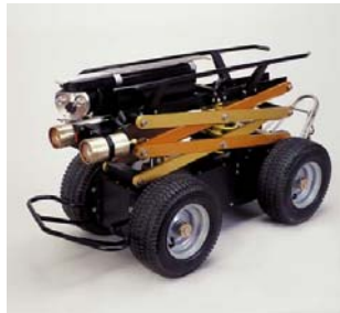
Storm Drain Tractor
