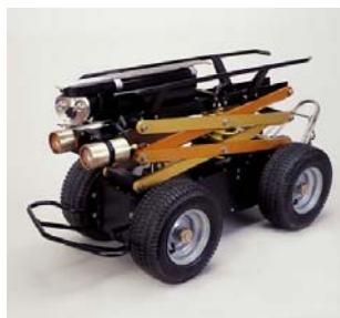
Storm Drain Tractor
