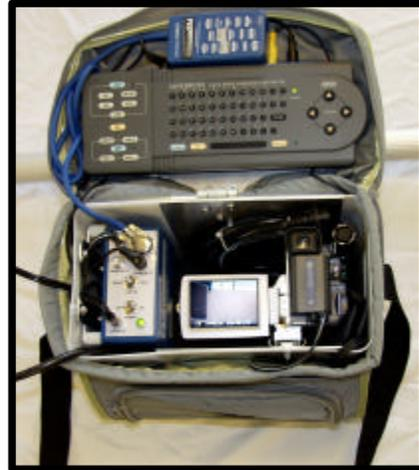
The **INVESTIGATOR Security Camera** is designed to provide clear video pictures in places unsafe or too small for human entry. The **INVESTIGATOR** comes with wheels to allow for ease of movement, and to support camera head to inspect hazards, contra band or structural defects under buildings and vehicles. The **INVESTIGATOR** is also well suited for use by municipal, HVAC and power and water departments in stacks, tanks, ducts, transformer vaults and most other confined spaces.
